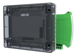
The unit is also available as a DIN Rail mountable version; both models feature an integral short-circuit isolator. The CHQ-DRC(SCI) utilises simple DIL switches for reliable addressing. A back box is also available (CHQ-BACKBOX) which, when used in conjunction with the CHQ-DRC(SCI), increases the IP rating to IP65.
